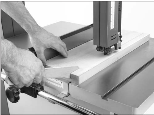
Figure 31. Ripping with a push stick.
